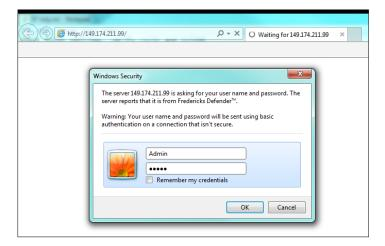
2.2.2 If the unit is connected to the network properly, the web page should be displayed. From here, data parameters can be viewed and changed along with current EthernetIP network settings.
